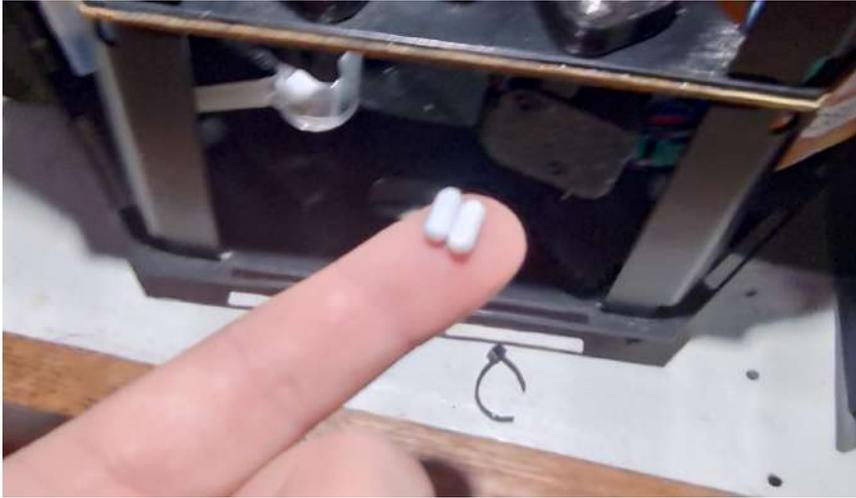
16. Install new magnetic stirrer head onto motor spindle.
