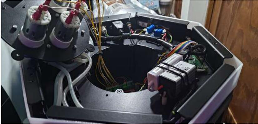
9. May need to remove Ethernet adapter. Loosen plastic nut closest to main board ~ 1 turn.
