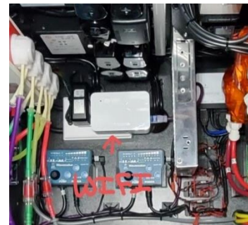
D-Link WIFI Extender DAP-1330 (Inside Cabinet Top Left Corner on Back Wall)
