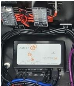
ILink Module ( ILNK 7 ) (Inside Cabinet Top Right Corner on Back Wall)
