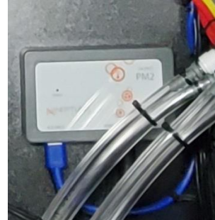
Tmpx4 Temp Probe connects to the PM Module (Inside Cabinet Bottom Left Corner on Back Wall)
