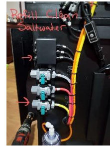
Refill ATO Connection Ports (Located on the Back of the Cabinet)
