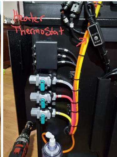
Heater Thermostat (Located on the Back of the Cabinet)
