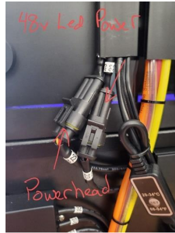
Quick Disconnects (Located on the Back of the Cabinet)
