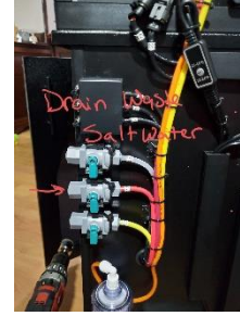
Drain Waste Saltwater Connection Port (Located on the Back of the Cabinet)
