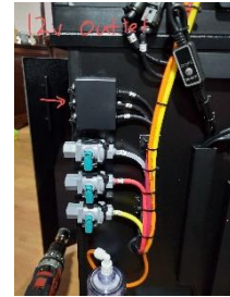
Refill ATO Connection Ports (Located on the Back of the Cabinet)
