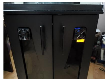
Cabinet Fans, CoolerGuys 60x20mm (Located in Front Cabinet Doors)
