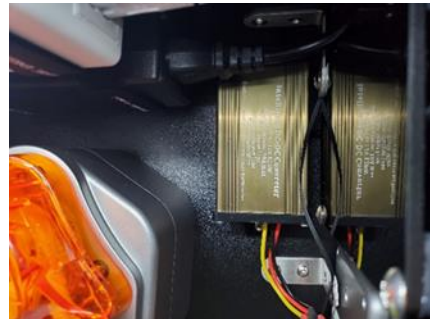
48v to 12v Converter (Located Inside Cabinet on Right Side at Top)
