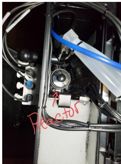
Reactor Top View (Located in the return pump chamber)
