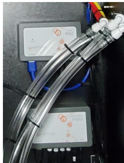
FMM_6 (Inside Cabinet Bottom Right Corner on Back Wall) 1. FLTR_1 (Filter Replace Sensor)
