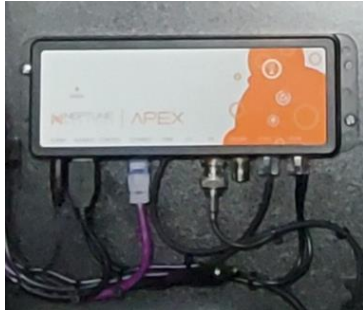
Tmp Temp Probe connects to the Apex Classic Base Unit (Inside Cabinet Bottom Left Corner on Back Wall)
