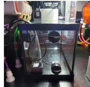
ATO Tank (Located Inside the Cabinet on the Left Side of the Shelf)
