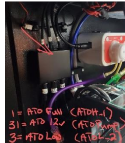
ATO Electrical Interface (Located inside cabinet on Left side wall towards the top)
