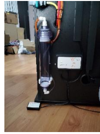
Co2 Scrubber (Located on the Back of the Cabinet)
