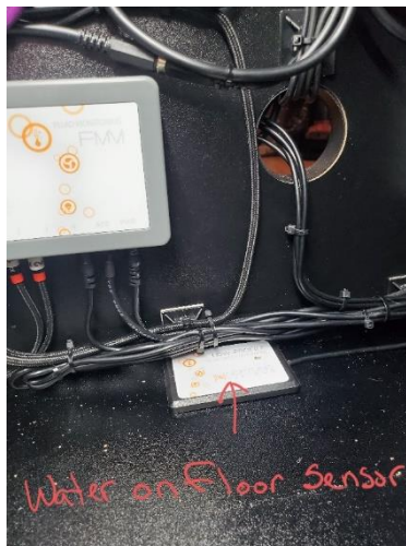
Water On Floor Sensor (2 Located Behind the Cabinet, 1 on the Left & 1 on the Right)
