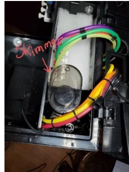
Coralife Biocube Skimmer 100538604 (Located in Right Rear Chamber)
