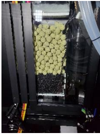
Mechanical & Wet/Dry Filtration (Located in Center Rear Chamber)
