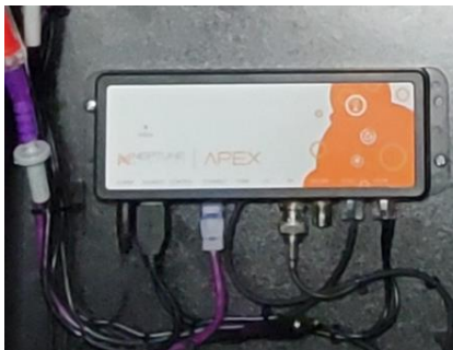
Apex Base Unit (Located Inside Cabinet Bottom Left Corner on Back Wall)
