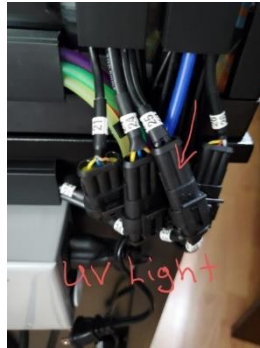
UV Light Quick Disconnect (Located on the Back of the Cabinet)
