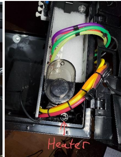
Vivosun Titanium 200 Watt Heater (Located in the Right Rear Chamber)
