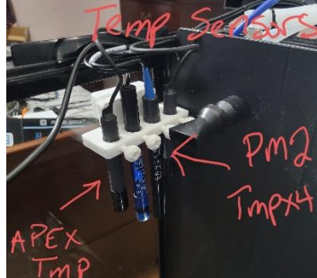
Temperature Probes (Inside Display Tank on Left Wall)
