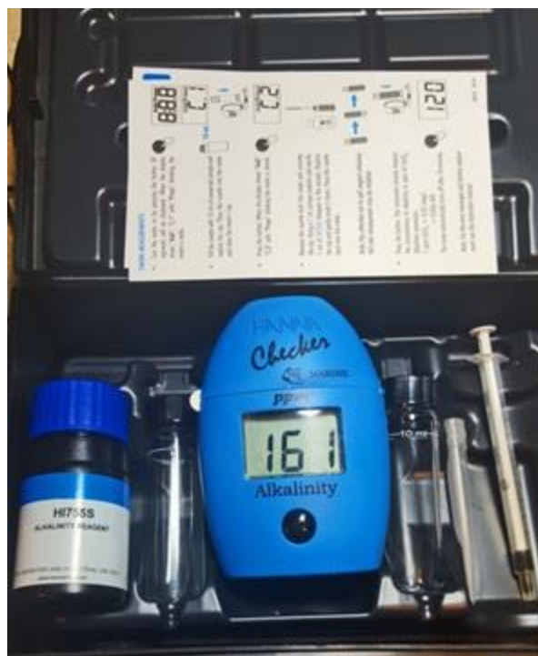
Figure One. The Hanna Checker colorimeter for determination of alkalinities typically found in reef aquaria. Everything is included for these determinations, including reagents sufficient for 25 tests.
