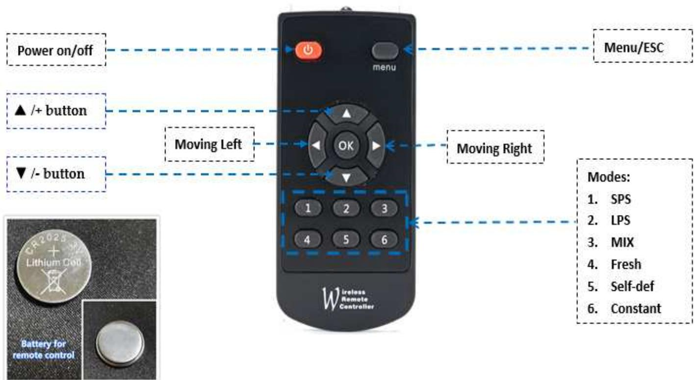
Note: Remote need install a lithium battery CR2025 3V before use.
